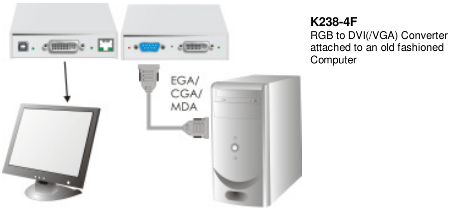
Figure 21 RGB to DVI(/VGA) Converter with optional EGA/CGA support, attached to an old fashioned Computer
